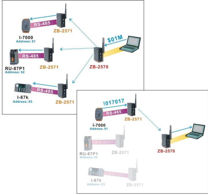
In some applications that the host controller needs to broadcast the data to all RS-232/RS-485 devices and these devices receive data only (no response), you can also use this mode.
