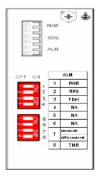
The plastic green colored contact power block (shown in the diagram to the left) is composed of six contacts and can be inserted and removed easily by hand to connect to the six pin terminal block receptor (male contacts located on the body of the The top two Converter). contacts (PWR) are designated for the primary DC input, while the middle two (RPS) are contacts for redundant DC input. The lower two contacts (ALM) are for connection to an external
