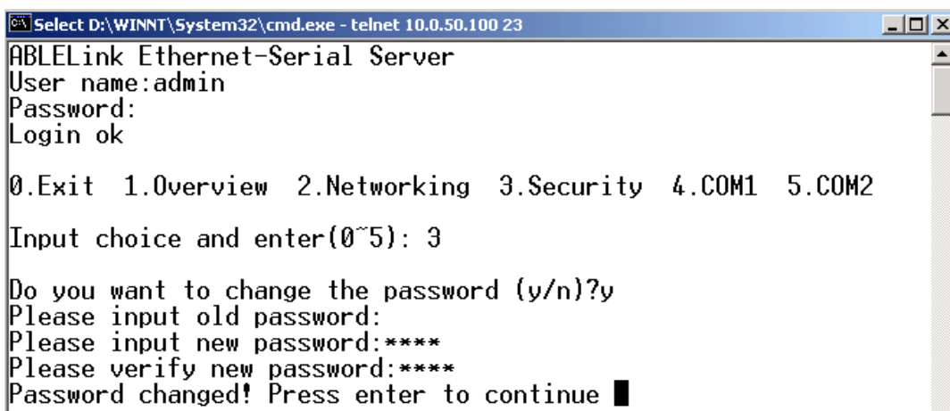
Fig. 13. changing password using Telnet
