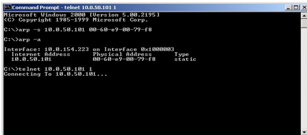
Fig. 34. Assigning a new IP address with ARP command
