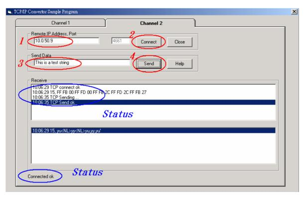
Figure 6.1 TCP test sample program in Visual B
