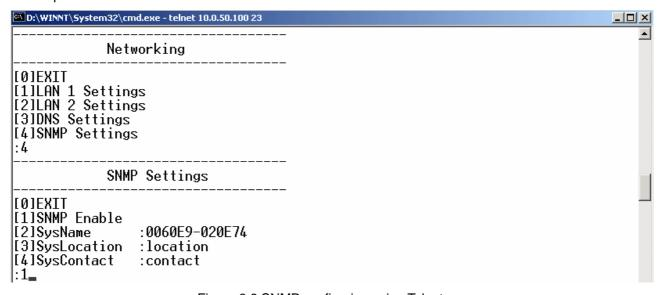
Figure 3.9 SNMP configuring using Telnet
