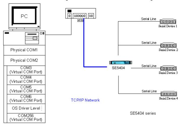
Figure 4.1 Virtual Com connection diagram
