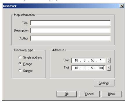
Figure 5.1 NetworkView-IP discovery parameters setup
