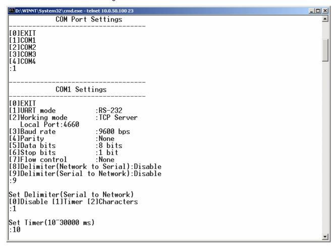
Figure 3.16 Setting packet delimiter timer-Packet delimiter timer
