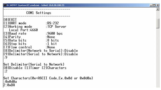
Figure 3.17 Setting packet delimiter-character pattern terminator
