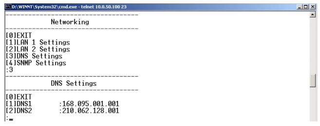
Figure 3.8 DNS configuring using Telnet
