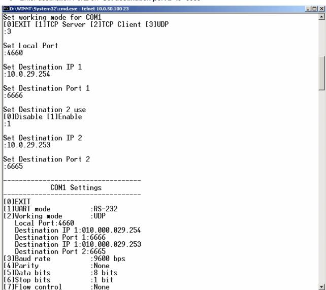
Figure 3.13 Link Mode-UDP client setup
