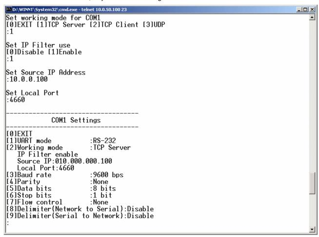
Figure 3.11 Working Mode-TCP server setup
