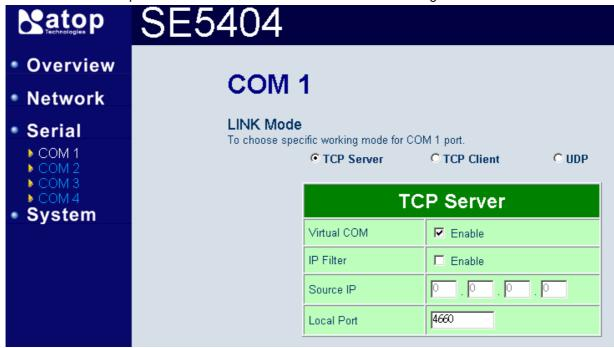
Figure 4.2 Enabling Virtual COM port
