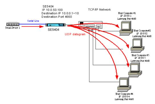
Figure 3.26 Data Transmission in a UDP Master(Client) Mode
