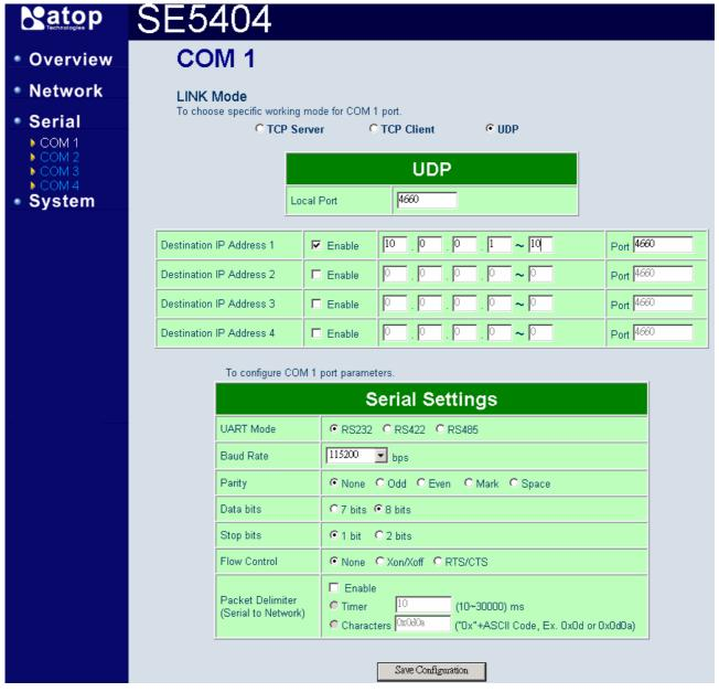
Figure 3.24 Com 1 setup -UDP mode
