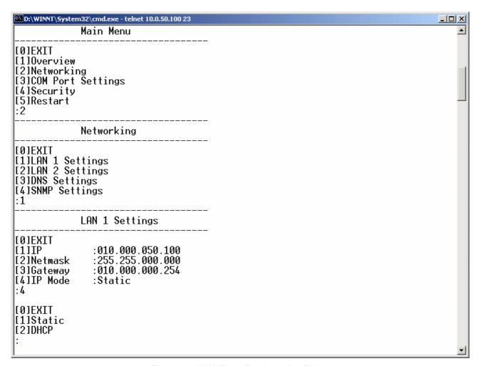
Figure 3.7 LAN IP configuring using Telnet
