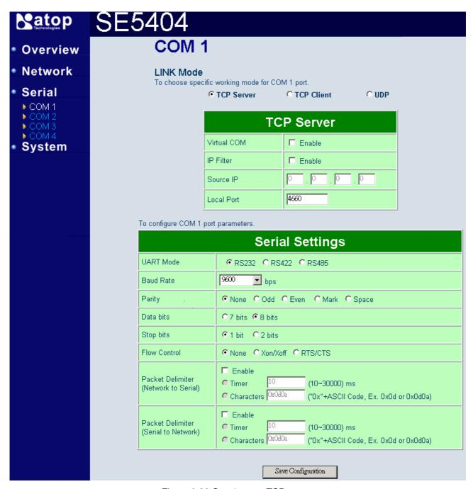
Figure 3.22 Com1 setup-TCP server
