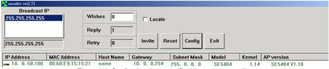
Figure 3.1. Configuring the static IP with monitor.exe utility
