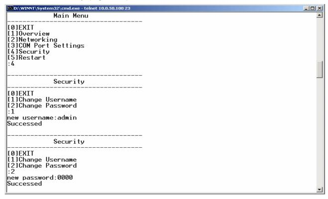
Figure 3.18 changing password using Telnet
