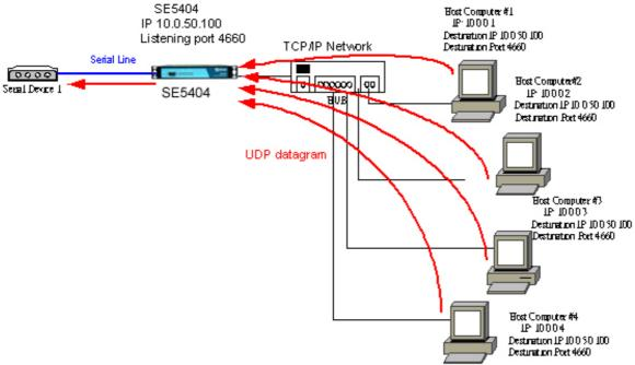
Figure 3.27 Data Transmission in a UDP Slave (server) Mode
