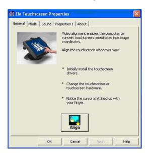
Click on the **Align** button. This launches the calibration program. The window shown below will open. Follow the instructions to calibrate the touchscreen.
