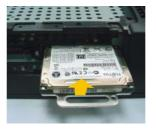
3. Secure the Hard Drive to the touchcomputer using the screw.
