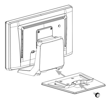
Pushing the stand plate toward the stand untill it is tight, then fasten the stand plate using captive screw.
