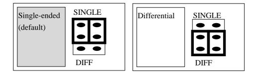
The A-821PGL/PGH offer 16 single-ended or 8 differential analog input signals. The JP3 select single-ended/differential. The user can not select single-ended and differential simultaneously.
