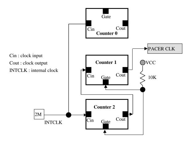
The counter1 and counter2 are all 16 bits counter. The counter 1 and counter 2 cascade as a 32 bits timer. This 32 bits timer is used as <u>pacer timer</u>. The software driver, A-822\_Delay(),
