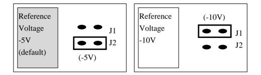
Select (-5V) : D/A voltage output = 0 to 5V (both channel) Select (-10V) : D/A voltage output = 0 to 10V (both channel) JP1 is validate only if JP2 select D/A internal reference voltage
