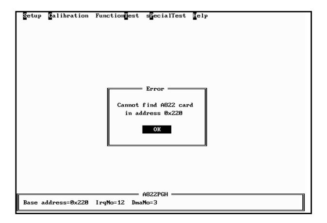
Although you can continue the A-822DIAG by press any key, it is recommended to correct this situation by setting the proper jumper setting. Because many operation in the A-822DIAG, the I/O base address is check firstly. And it don't work if the error occurs
