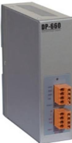
DP-660 is a **65** watts, universal input switching mode power supply. It is with **24V/5V** output options. DP-660 is intended for power device like motor or solenoid application. Built in +5V 3T-regulator for DP-660 is for if there is a logical control circuit.
