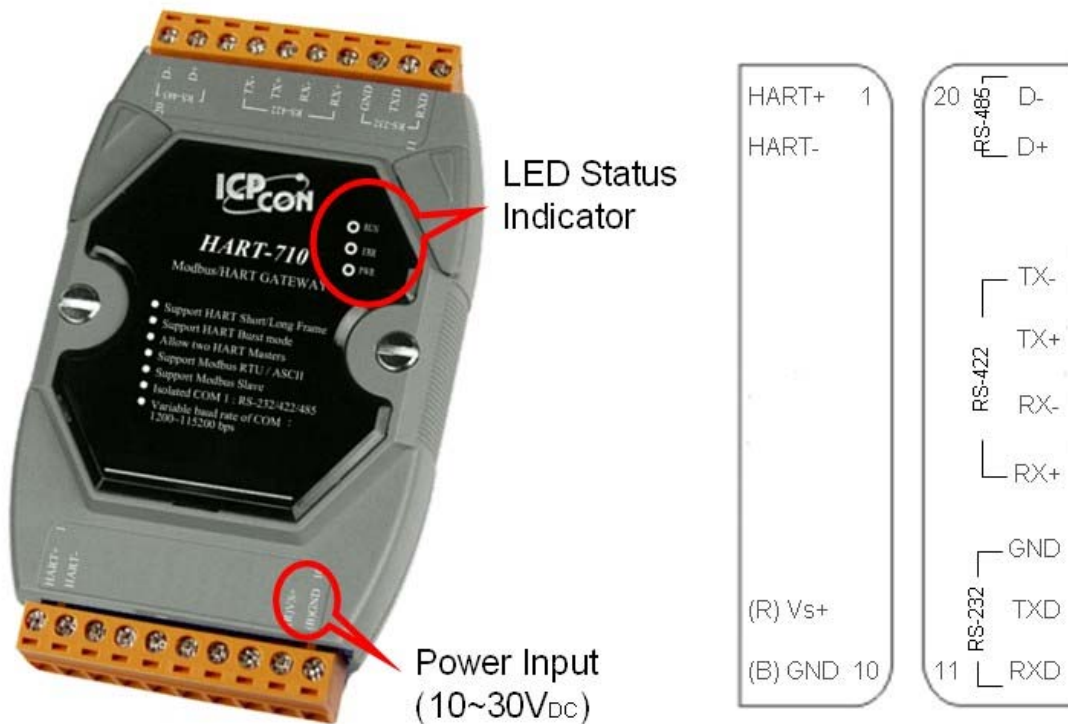
Figure 3: Pin assignment of HART-710
