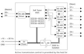
outbound messages from the Master input. All channels transmit simultaneously.
