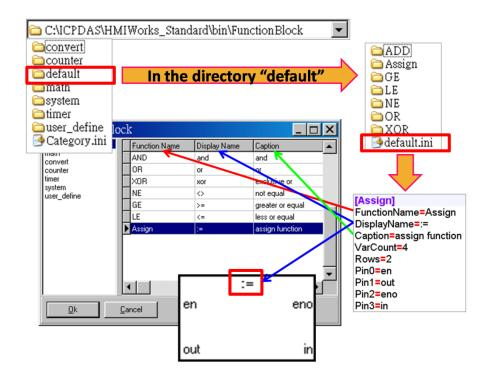
3. Double click on the "Assign" to use it in the Ladder Designer. The Ladder Designer uses the logics defined in the file "FB.hsf" in the sub-directory "Assign". FB.hsf is based on the C language. The following figure explains what FB.hsf of the "Assign" function does.
