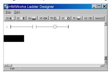
Double click the contact input of the first rung in the **Ladder Designer** window. Then the "Select variable" dialog box is displayed. Choose the variable to associate with the contact input.
