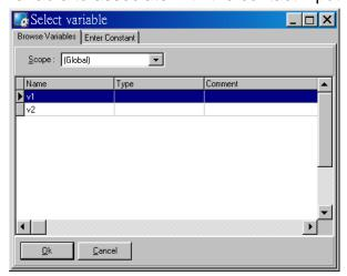
Here, we select variable v1 to associate the contact input. Repeat the same procedure to associate v2 with the coil output.
