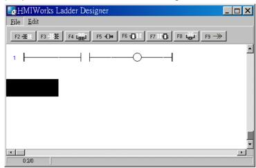
To delete a rung, move the cursor to the starting point of the rung and then press "Delete" key.
