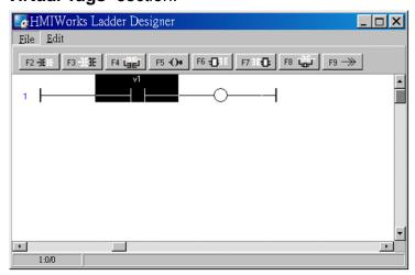
Insert a new contact input in the left of the cursor (F2) Move the cursor to the "v1" contact input and then press F2. And to make things clear, associate variable "v2" to the newly-inserted contact input.
