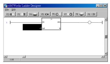
Set "v2" to "in" of "Assign" function in the same way. Finally, set "v3" to the coil output.
