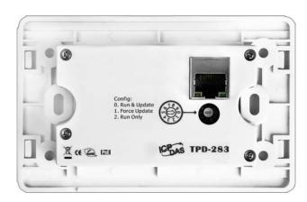
On the back panel of a TPD-283 device, configuration modes can be found.
