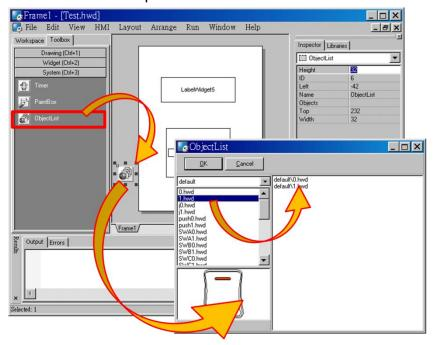
Make the CheckBox component refer to the ObjectList component by setting the property "RefObject" to the ObjectList component. Now toggling the states of the CheckBox component becomes the switching of the pictures in the ObjectList component.
