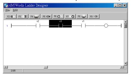
Insert a new contact input which is parallel to the cursor (F4) Move the cursor to the "v3" contact input and then press **F4**.
