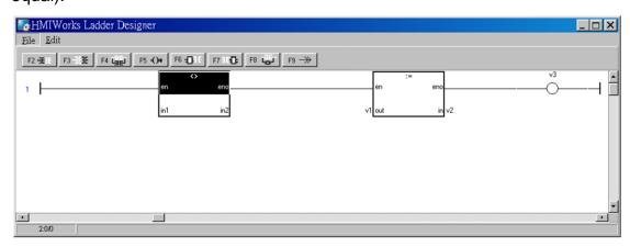
Insert a new function block in the right of the cursor (F7)
