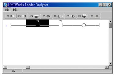
Insert a new contact input in the right of the cursor (F3) Move the cursor to the "v2" contact input and then press **F3**. Associate variable "v3" to the newly-inserted contact input.
