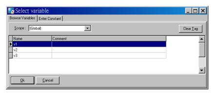
Double-click on the variable in the list to assign the variable to "out". For example, we double-click on the variable "v1" and set to "out" of "Assign" function.
