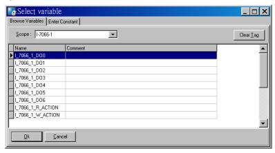
Double click on the tag Name you want to associate with the widget. Then you can see the tag is associated with the widget (that is, the Slider for example) by setting the property TagName to the name of the tag.
