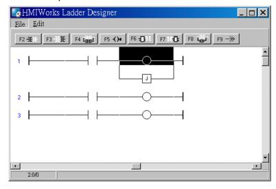
3. Double click on the starting point of the third rung to add a label "Test\_Label" to it.
