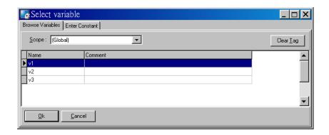
For example, we double-click on the variable "v1" and set to the contact input. v1, v2 and v3 are the variables set by "New Virtual Tags". Refer to the "New Virtual Tags" section.
