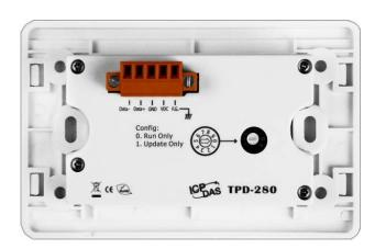
On the back panel of the TPD-280 device, configuration modes can be found. Use the rotary switch to set the configuration mode.
