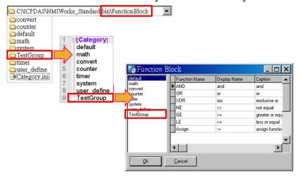
2. Go to the directory "TestGroup", create a .ini file of the exactly same name as that of the group, that is, "TestGroup". Create a sub-directory of the "TestGroup" directory and we may call the sub-directory "TestFunction". Finally, define a new function, "TestFunction" in the file "TestGroup.ini".
