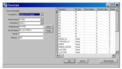
Step by step specify or fill each field and click the **OK** button to import tags. Finally, check these imported tags in the Workspace.
