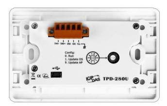
Except the TPD-280 and the TPD-283 devices, users can find out the same definitions of the configuration modes on their back panels for other devices in the TouchPAD series. We use the rotary switch to set the configuration mode.
