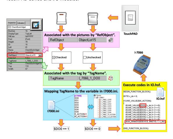
**Note**: The TagName property takes effect only in the programming type Ladder. (It's easier in programming type "Standard C". Control the I/O by using API function, dcon WriteDO, in the event handler of the CheckBox.)
