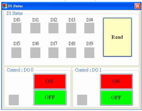
The function is used for controlling DO and reading the status of DIs:
