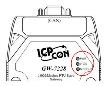
Figure 2-17: LED position of the GW-7228
