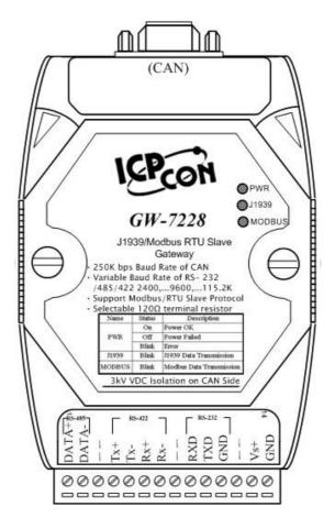
Figure 2-1: Hardware externals of the GW-7228
