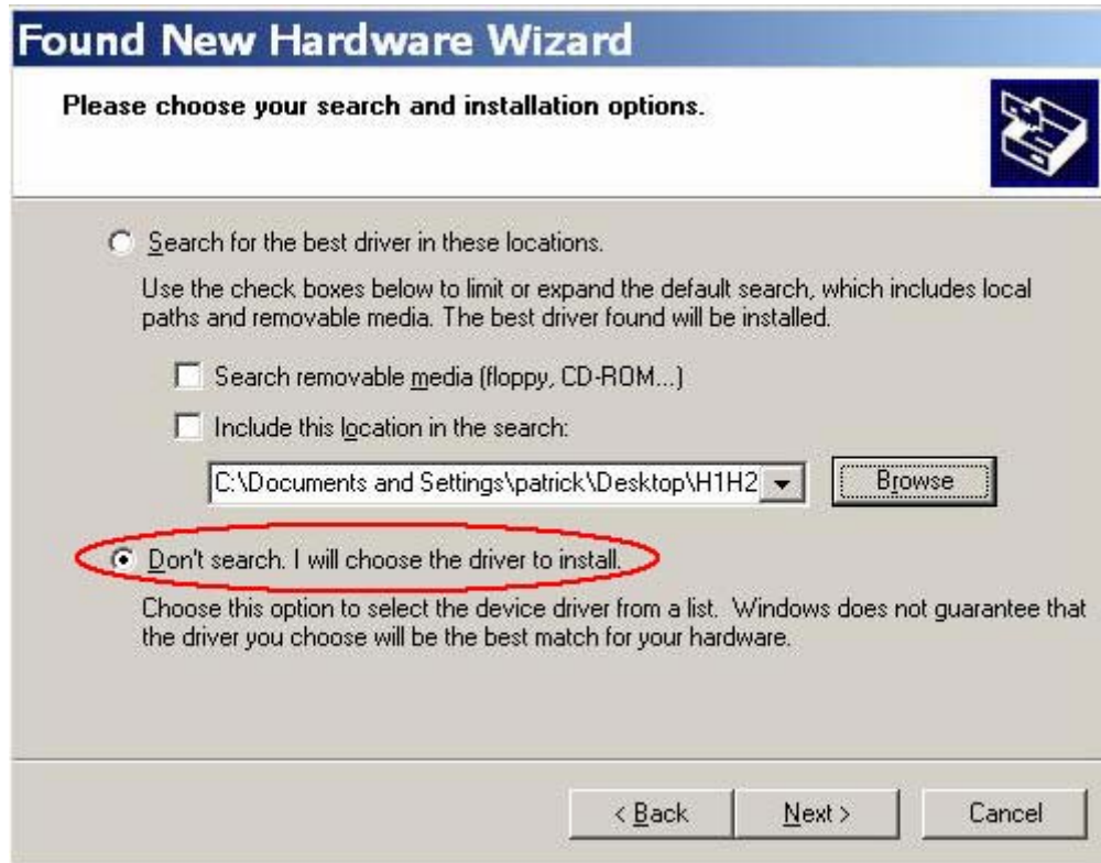
Figure 6-4: Driver Installation of I-7565-H1/H2 (1) (4) When the Figure 6-5 shows, click “Next” button and the other steps are the same with those in chapter 3.
