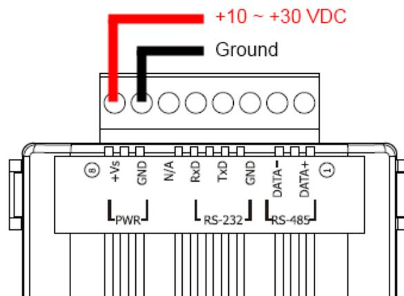
Fig. 2-10: Wire connection for the power.
