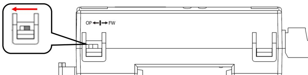
Fig. 2-14: Push the switch to “OP” mode
