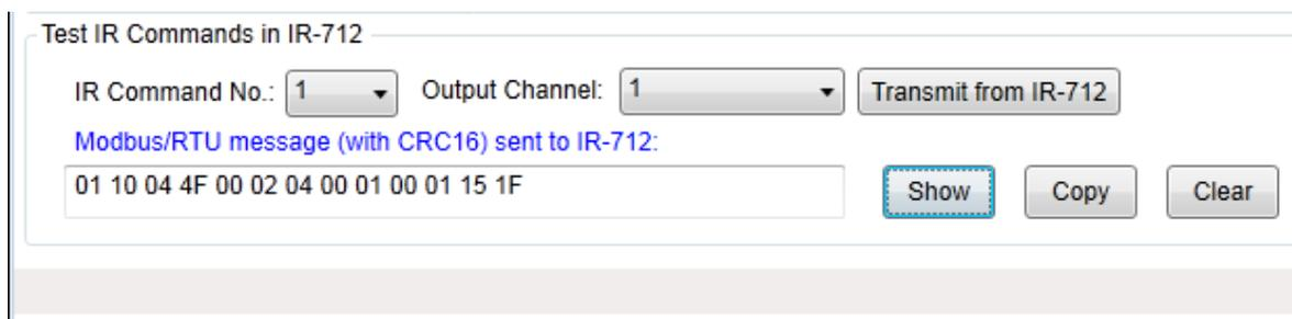
Fig. 3-18: Test IR commands saved in IR-712.
