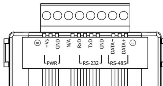
Fig. 2-3: Screw terminal connector
