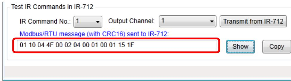
Fig. 4-8 Test the IR commands saved in the IR-712
