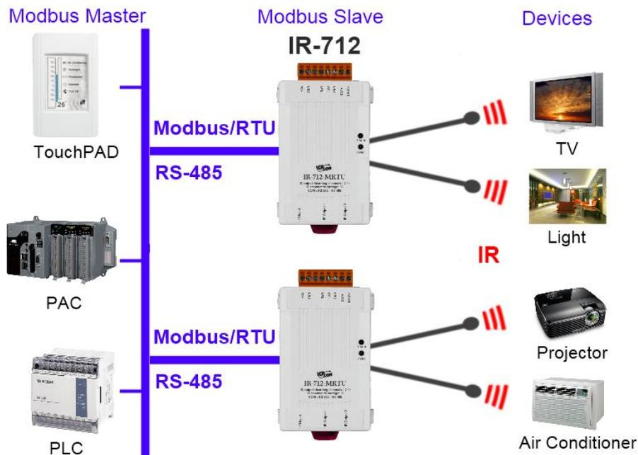
Fig. 1-1: IR-712 application architecture.
