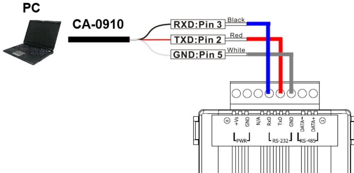
Fig. 2-6: Wire connection between PC and IR-712 using CA-0910.
