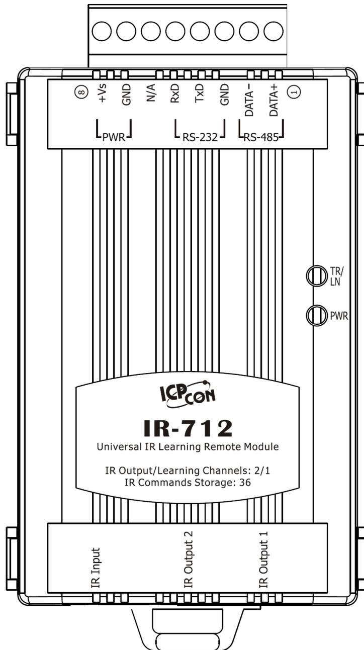
Fig. 2-1: The front view of the IR-712.
