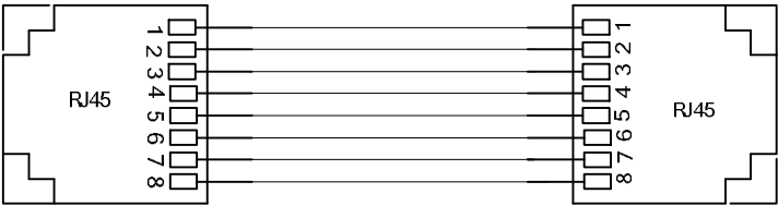
Figure.A-2 Order of Straight-through Cable
