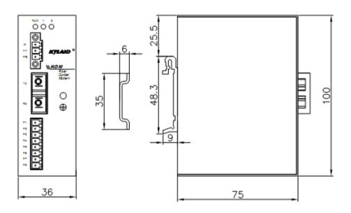
Figure 9 Dimension diagram of DIN-rail installation
