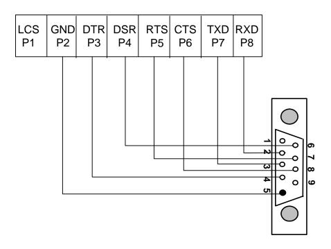
Figure 6: KOM200-V.24 Interface Diagram
