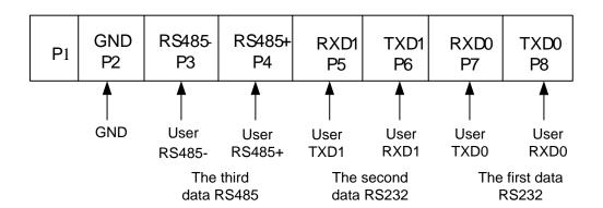
Figure 3: KOM200-485/232 KOM200-485/232A Interface Diagram
