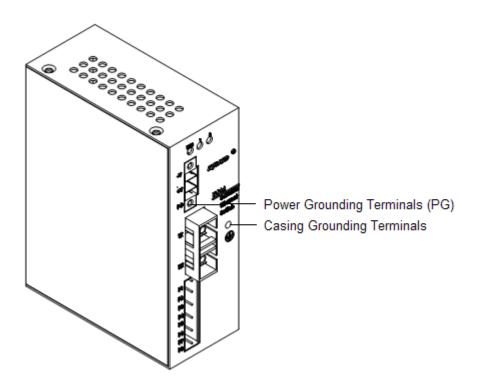
Figure 7: Device grounding
