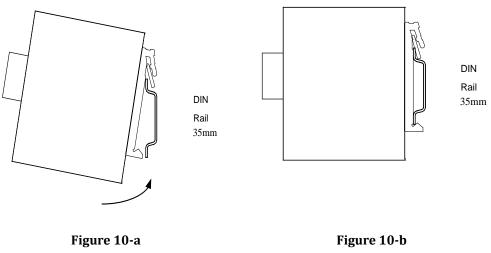
Figure 10 Install KOM300 into Rail
