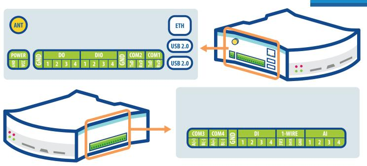
iMod 9500 M3 - Industrial Embedded Computer based on the Linux system
