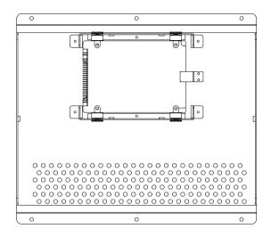
Step 3: Assembly the damper bracket
