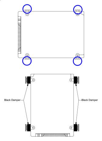
Step 2: Assembly the HDD chassis
