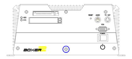
Step 2: Unfasten the screw on the front panel.
