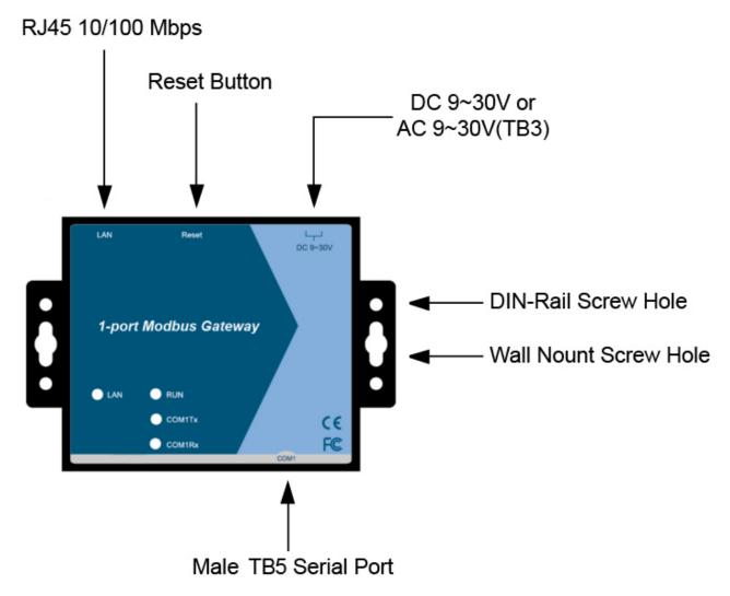
Figure 2.2 MB5001C-Sis interfaces
