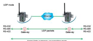
Serial Data exchange via tunnelling mode
