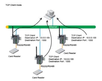
Fig 7. TCP Client in Virtual COM Mode
