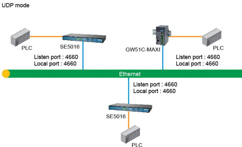
**Fig 9.** Work mode by UDP Connections
