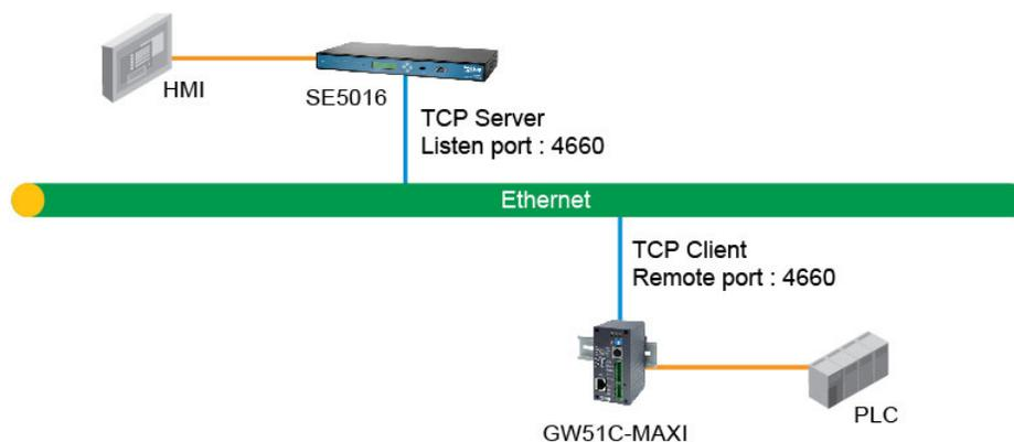
**Fig 7.** Work mode by TCP Connections
