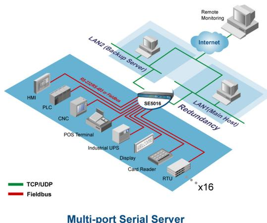
Fig 1. Topology of SE5008/5016 Multi-application Connectivity
