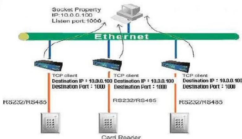
Fig 5. TCP Client of Virtual COM Operation Mode
