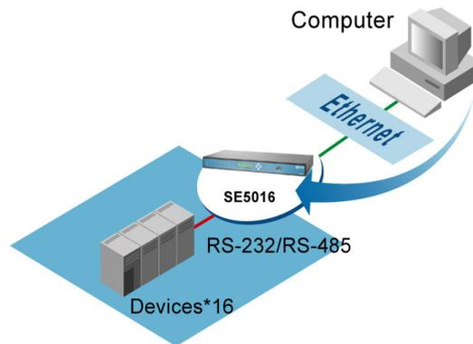
Fig 2. TCP Server of Virtual COM Mode's Connectivity
