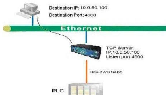
Fig 3. TCP Server of Virtual COM Operation Mode
