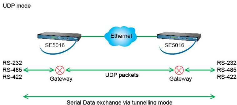
**Fig 8.** UDP mode for Tunneling mode
