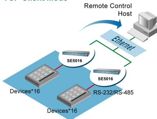
Fig 4. TCP Client of Virtual COM Mode's Connectivity
