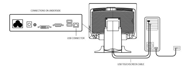
Connect one end of the **USB cable** to the rear side of the computer and the other to the LCD monitor.
