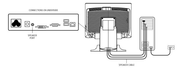
Connect one end of the **speaker cable** to the speaker port in the computer and the other end to the port in the monitor.
