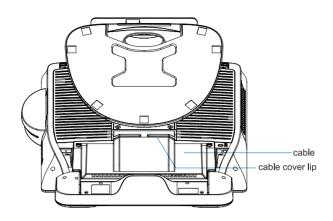
Then you have attached all the cables to the monitor, gently bring all the cables toward the standard so they fit under the cover lip.
