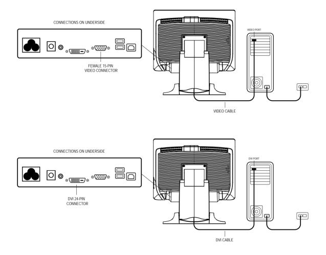
Connect one end of the **video cable** to the rear side of computer and the other to the LCD. Tighten by turning the two thumb screws clockwise to ensure proper grounding. You can select DVI video cable or D-SUB15 video cable.
