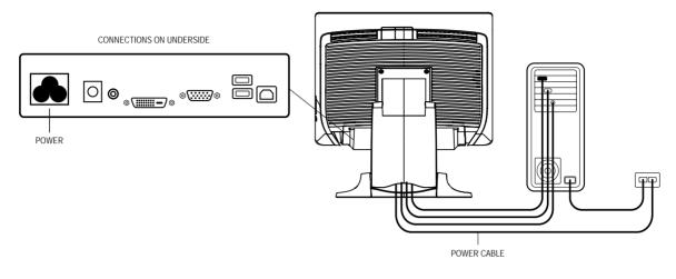
Connect one end of the **power cord** to the monitor and the other end to wall. Connect the power cable to the power port in the monitor.
