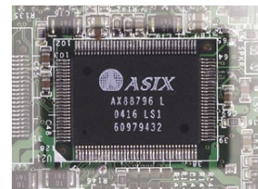
ASIX AX88796L 10/100Mbps Ethernet Controller
