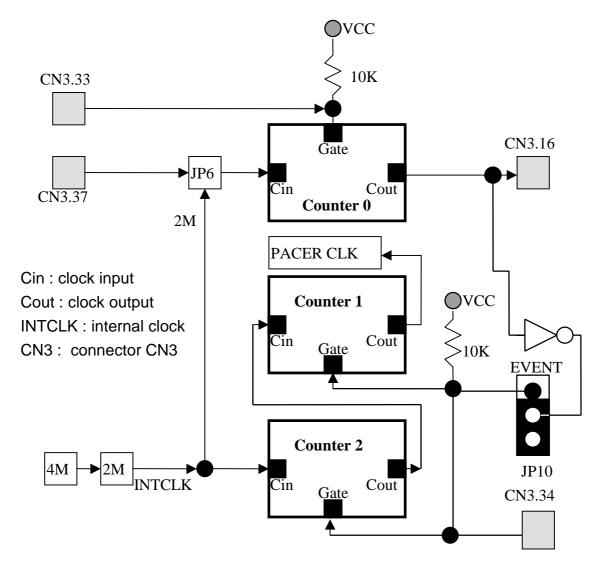
The counter0, counter1 and counter2 are all 16 bits counter. The counter 1 and counter 2 cascade as a 32 bits timer. This 32 bits timer is used as <u>pacer timer</u>. The software driver, A826\_Delay(), use counter 0 to implement a machine independent timer for settling time delay. If user doesn't use A826\_Delay(), the counter0 can be used as a general purpose timer/counter.
