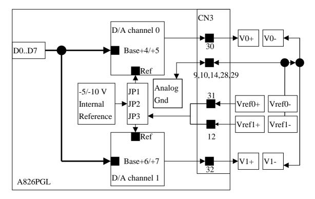
NOTE : The DA output latch registers are designed as "double buffer" structure. <u>The</u> <u>user must send the low byte data first, then send the high byte</u> <u>data to store the DA 12 bits digital data</u>. If the user only send the high byte data , then the low byte data will be still the previous value. Also if the user send high byte first then send low byte, the low byte data of DA is still hold in the previous one.
