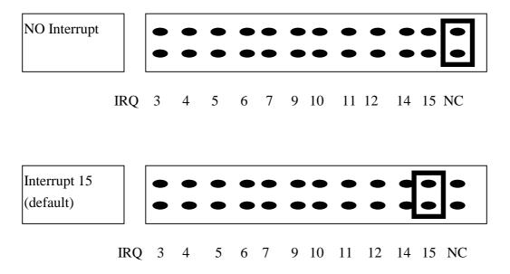
The interrupt channel <u>can not be shared.</u> The A826 software driver can support 8 different boards in one system but only **2 of these cards** can use interrupt transfer function.
