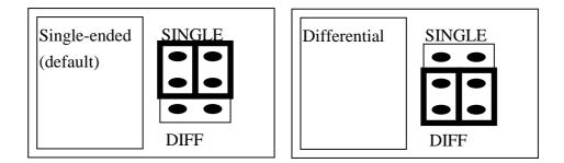
The A-826PG offer 16 single-ended or 8 differential analog input signals. The JP4 select single-ended/differential. The user can not select single-ended and differential simultaneously.
