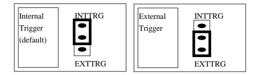
The A-826PG supports two trigger type, **internal trigger** and **external trigger**. The external trigger signal comes from **ExtTrg, CN3 pin 17**. There are two types of internal trigger, **software trigger** and **pacer trigger**.
