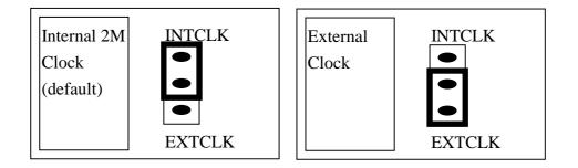
The A-826PG has 3 independent 16 bits timer/counter. The cascaded counter1 and counter2 are used as **pacer timer**. The counter0 can be used as a user programmable timer/counter. The user programmable timer/counter can select **2M internal clock** or **external clock ExtCLK, CN3 pin 37**. The block diagram is given in section 2.6. The clock source must be very **stable.** It is recommended to use internal 2M clock.
