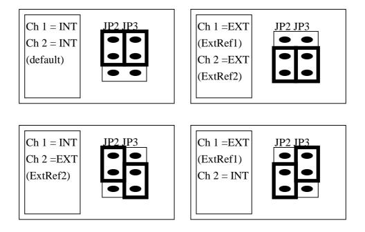
If JP2/JP3 select **internal reference**, then JP1 select **-5V/-10V** internal reference voltage. If JP2/JP3 select **external reference**, then **ExtRef1**, **CN3 pin 31**, is the external reference voltage for DA channel 1. and **ExtRef2**, **CN3 pin 12**, is the external reference voltage for DA Channel 2. If user provides AC +/- 10V external reference voltage, the D/A output voltage may be AC -/+ 10V
