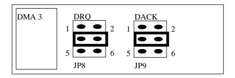
**The DMA channel can not shared.** The A826 software driver can support 8 different boards in one PC based system, but only **two of these boards** can use DMA transfer function.
