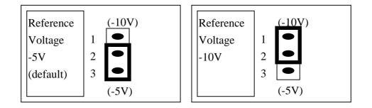
Select (-5V) : D/A voltage output = 0 to 5V (both channel) Select (-10V) : D/A voltage output = 0 to 10V (both channel) JP1 is validate only if JP2 /JP3 select D/A internal reference voltage
