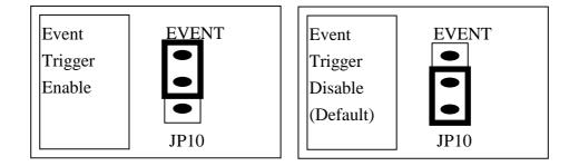
Both of <u>the machine independent time</u>r and <u>the event trigger controller</u> use timer/counter 0. Only one of these two function can be implemented. <u>So the user can not</u> <u>use both function at the same time.</u>
