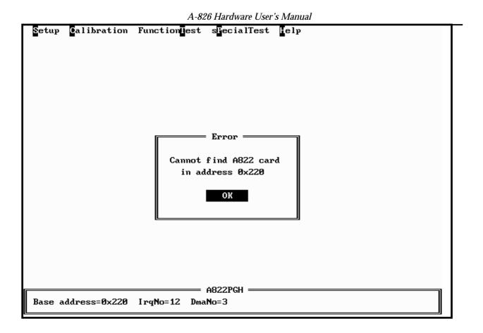
Although you can continue the A82XDIAG by press any key, it is recommended to correct this situation by setting the proper jumper setting. Because many operation in the A82XDIAG, the I/O base address is check firstly. And it don't work if the error occurs
