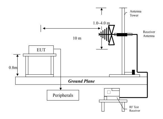
The equipment under test was placed on the top of rotation table 0.8 meter above ground plane.
