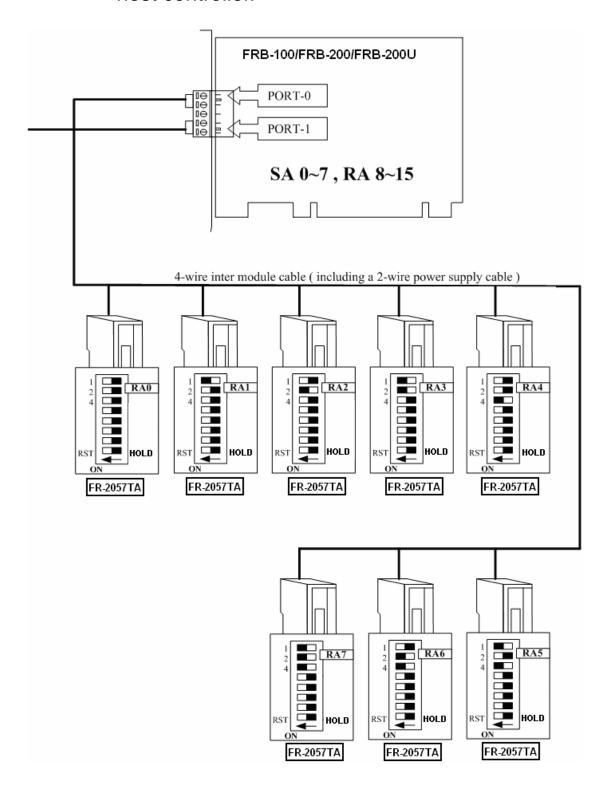
Figure 2.6 PCI interface FRnet card and distributed IO modules
