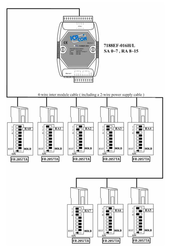
Figure 2.7 Embedded controller and distributed IO modules
