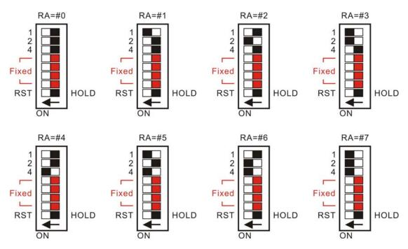
Figure 2.5 Receiver address setting.
