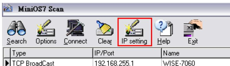
Figure 2-3 : IP Setting button on MiniOS7 Scan
