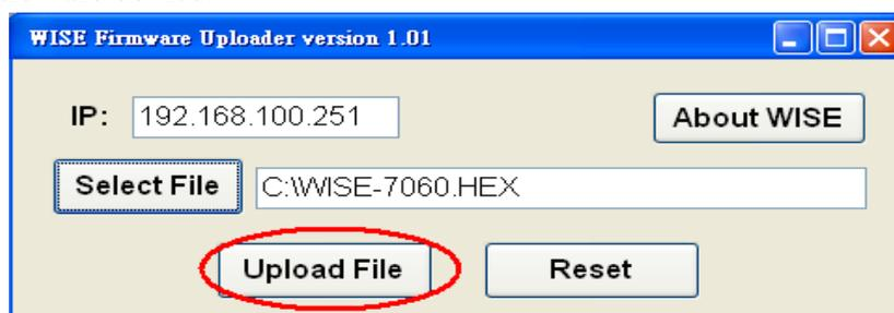
Figure 10-12 : Upload firmware
