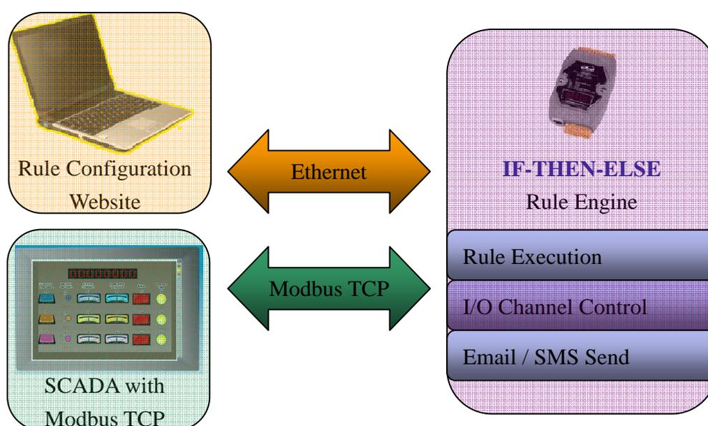
Figure 1-1 : WISE system architecture
