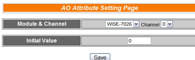
The screenshot shows the AO Attribute Setting page. At the top is an orange header bar with the text "AO Attribute Setting Page". Below this is a "Module & Channel" section with a dropdown menu showing "WISE-7026" and a "Channel" dropdown menu showing "0". Below that is an "Initial Value" section with a text input field containing "0". At the bottom center is a "Save" button.
