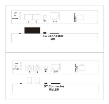
The Wavelength used is 850nm. The series also support MM(multimode) fiber cables. The recommended MM cable is 62.5/125µm.
