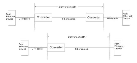
**Important rule:** When a connection is established, make sure the devices located at both ends of the path are configured and operated using the same duplex mode and the maximum distance must comply with IEEE 802.3u specifications.
