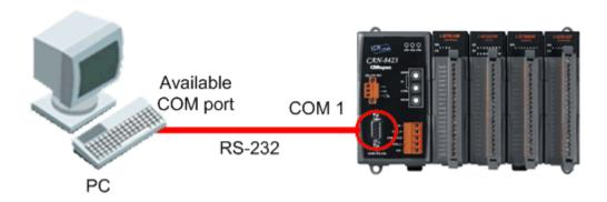
Step 1: To turn off the CAN-8423 is the beginning. Then, users can set the "Baud" rotary switch of CAN-8423 to 9. Then, turn on the CAN-8423.
