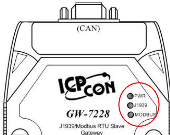
Figure 2-17: LED position of the GW-7228
