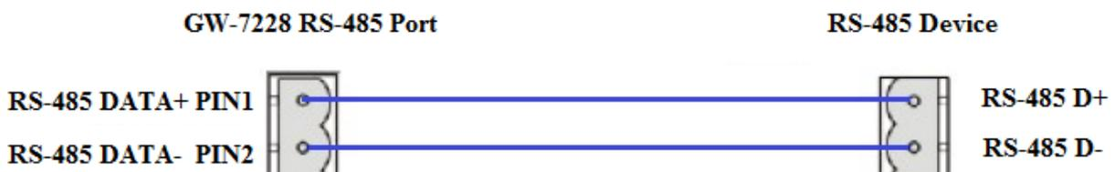
Figure 2-7: RS-485 Wire Connection
