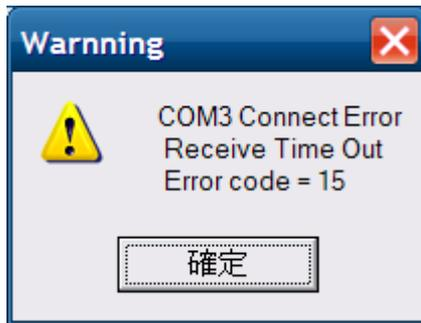
Figure 3-3: COM Receive Time Out Error Screen
