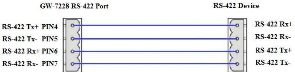
Figure 2-6: RS-422 Wire Connection
