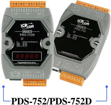
Programmable Serial-to-Ethernet Device Servers
