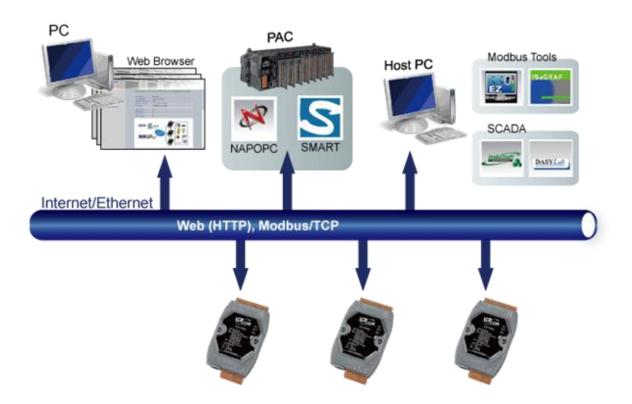
The ET-7002/PET-7002, a web-based Ethernet I/O module, features a built-in web server, which allows configuration, I/O monitoring and I/O control by simply using a regular web browser.
