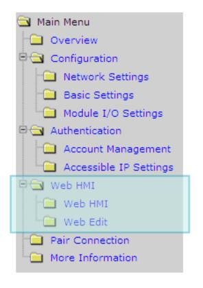
**Web HMI:** Links to the I/O monitor page that allows you to monitor and control the I/O status on ET-7002/PET-7002 module remotely.
