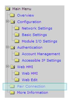
This pair connection function is a particular feature of ET-7002/PET-7002 that can enable a pair of DI-to-DO via Modbus/TCP. With pair connection function enabled, ET-7002/PET-7002 modules can poll the status of remote DI devices using the Modbus/TCP protocol and then continuously write to its DO channels in the background.
