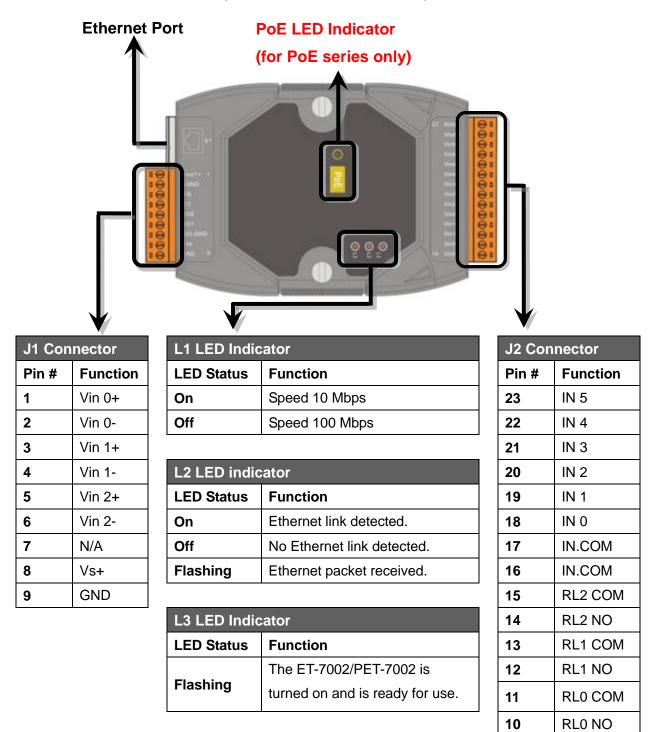
The ET-7002/PET-7002 front panel contains the Ethernet port, connectors and LEDs.
