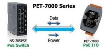
When using PET-7002 module, you can choose ICP DAS "PoE" switch – "NS-205PSE" as the power source, NS-205PSE automatically detects the connected devices whether they are PoE devices or not. This mechanism ensures NS-205PSE to work with both PoE and non-PoE devices coordinately at the same time.
