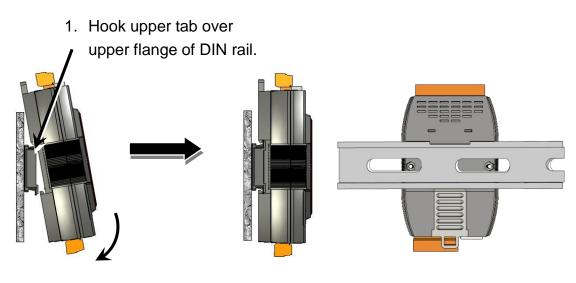
2. Tilt the module toward DIN rail until it snaps securely to DIN
