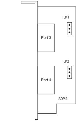
Figure 2.5 ADP-9 Board LAYOUT (For PISO-CAN400/PISO-CAN400U Only)
