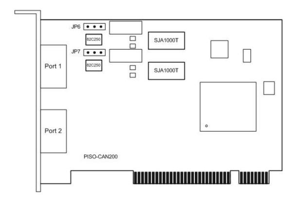
Figure 2.1 PISO-CAN 200 Board LAYOUT
