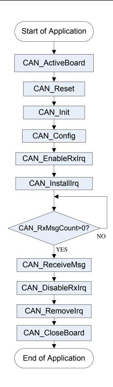
Figure 4.3 Flow Chart "Receive CAN Massage with IRQ"
