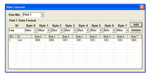
■ Software ID Mask: If users don't want to show some message with specific ID on the reception list, the ID mask function is useful for that. As following figure, users can set maximum 20 different ID message in the ID mask list. Afterwards, if the CAN port receives the message with the ID set in ID mask list, the CAN message will not shown in the reception list.
