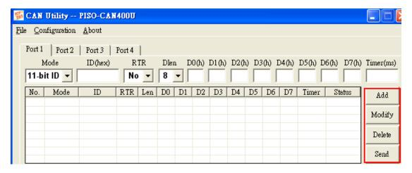
Add Button: User can key in the CAN message into the text boxes above the transmission list. Then click add button to insert this CAN message into transmission list. The transmission list can include maximum 20 CAN messages. After adding the message into transmission list, users can send this message to CAN network by using Send button.
