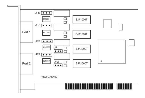
Figure 2.2 PISO-CAN400 Board LAYOUT
