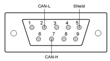
Figure 2.9 9-pin D-sub male connector
