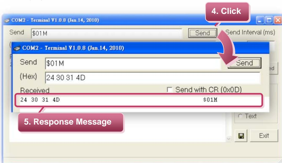
4. If the test is successful, then your COM port program should now be able to work with this Virtual COM Port.
