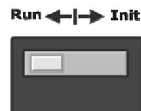
In the tDS-700 series, the operating mode Switch is in the Run position by default. When updating the tDS-700 firmware, the switch needs to be moved from the Run position to the Init position. The Switch must be returned to the Run position after the update is complete.
