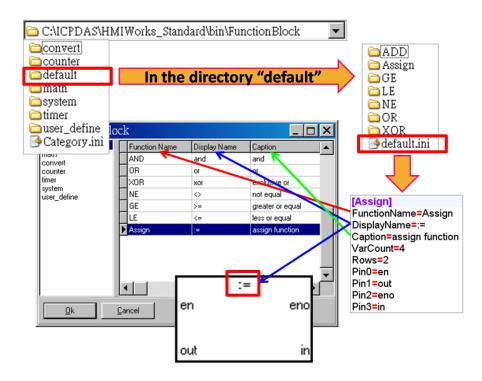
Double click on the "Assign" to use in the Ladder Designer. Ladder Designer uses the logics defined in the file FB.hsf in the sub-directory "Assign". FB.hsf uses C language. Following figure explains what FB.hsf of "Assign" does.
