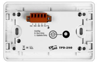
In the back of the TPD-280, configuration modes can be found. Use the rotary TouchPAD User Manual, version 1.0.9. Last Revised: September 2011 Page: 37
