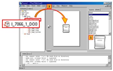
HMIWorks does the followings to build the relationships between TouchPAD and I/O modules.
