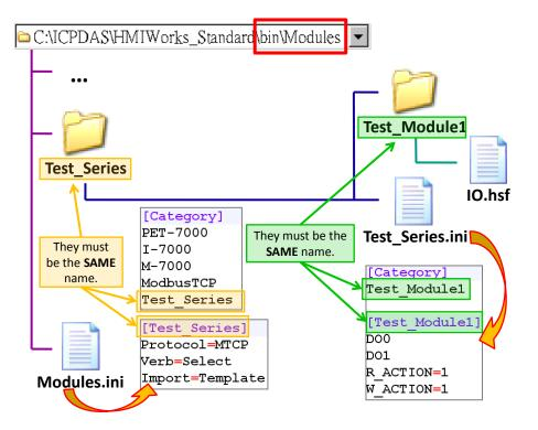
In the directory, "[HMIWorks install path]\bin\Modules\", create a new I/O series directory whose name is "Test\_Series" and be sure to update Modules.ini to notify HMIWorks that there is a new I/O series called "Test\_Series". As the figure shows, the series directory name and the name in the Modules.ini must be **the same**.
