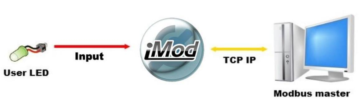
In this example the application counts the USER\_LED changes and saves the amount of the changes in the iMod register.
