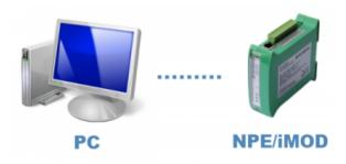
Direct connection between a computer and the device requires additional network interface configuration. The device should be connected directly to a computer with an Ethernet network cable.
