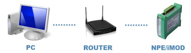
Another method is connecting the device to a local area network (LAN). If a router in the network has the DHCP (Dynamic Host Configuration Protocol) service active, the device IP address will be randomly assigned after start. In order to improve searching for the addresses assigned to devices in the local area network the SearchNPE application has been created.
