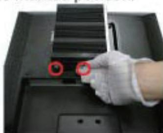
3. Lock the chassis to the chassis stand by tightening up the two screws in the marked position.
