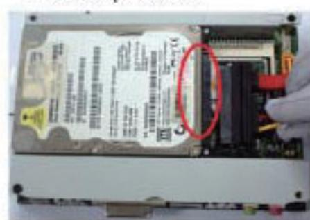
6. Plug the cable to the SATA power connector and SARA connector.
