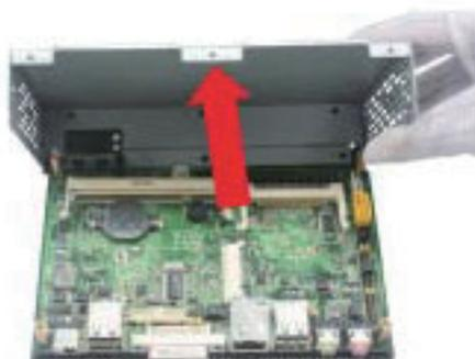
3. Lift the cover upwards to open the chassis.
