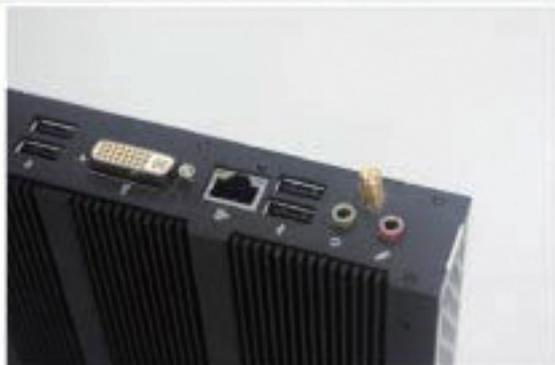
5. Push the antenna connector from inside of the chassis into the back panel RF slot.
