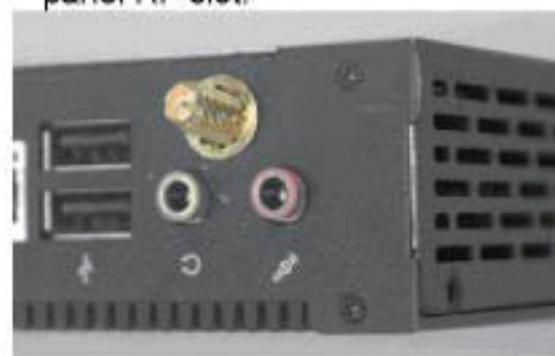
7. Put the washer into the antenna connector at first.
