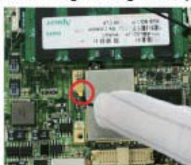
4. Press the metal hat on the end of the antenna string to the antenna slot on the card as shown.
