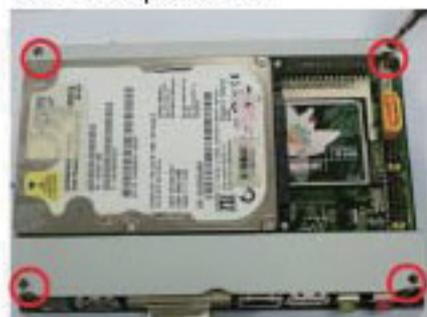
5. Lock the racks to the board by tightening up the screws in the marked position with a screwdriver.
