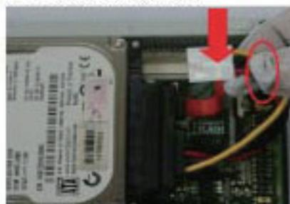
7. Plug the other end of the cable to SATA power connector and SATA connector onboard.
