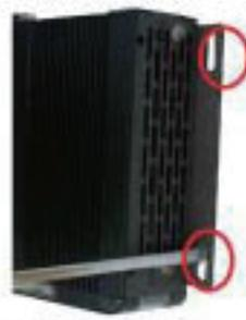
4. Tightening the other two screws in the marked position on the other rack.
