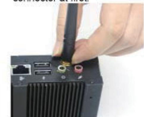
9. Connect the external WiFi receiver to the antenna connector on the rear panel.
