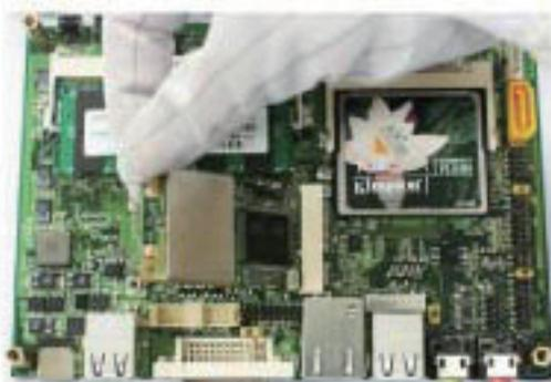
2. Insert the gold-figure side of the compatible mini-PCI-E card into the slot at a 30 degree angle and press down.
