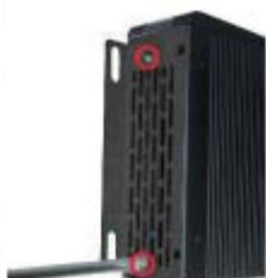
1. Install wall mount rack to the system by tightening two screws in the marked position.
