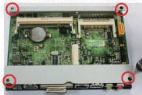
1. Remove the screws in the marked position with a screwdriver.
