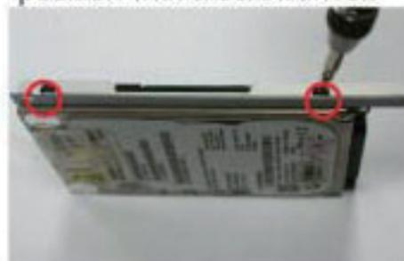
3. Lock the SATA hard disk to one of the racks by tightening the screws in the marked position.
