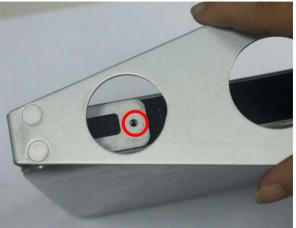
2. See to it that the marked tiny round space and the screw hole in on the chassis are in the same place.
