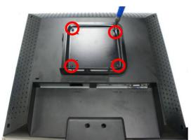
1. Attach the chassis rack to the back of monitor by tightening up the screws in the marked position.
