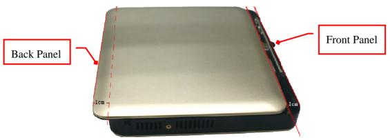
3. Place the removable cover upon the chassis. See to it that the left and right edges of the cover should be parallel to those of the chassis and there should be a distance of about 1 cm left between the front edge and the front panel of the chassis as the photo shows.
