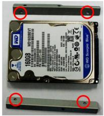
The SATA hard disk and the hard disk racks (see to it that the marked screw holes on rack and the corresponding holes on both edges of HDD).
