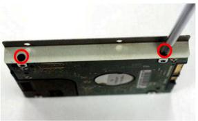
Lock the SATA hard disk to the other rack by tightening the screws in the marked position.
