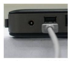
USB Connector: There are 3\*USB connectors on rear IO panel (one is USB/E-SATA shared connector that functions according to device connected) and 2\*USB connectors on the front panel to connect USB mouse, keyboard and other USB storage devices to the system.
