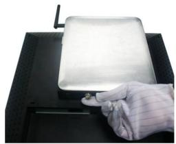
4. Lock the chassis to the rack by tightening up the screw in the marked position.
