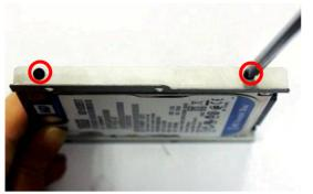
3. Lock the SATA hard disk to one of the racks 4. by tightening the screws in the marked position.
