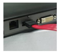
USB/E-SATA Shared Connector: The function of this connector depends on different device connected to this connector through different cable.
