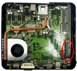
1. Locate HDD connector on the motherboard as the photo shows.
