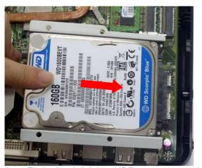
5. Fit the hard disk into HDD connector on the motherboard in this direction.
