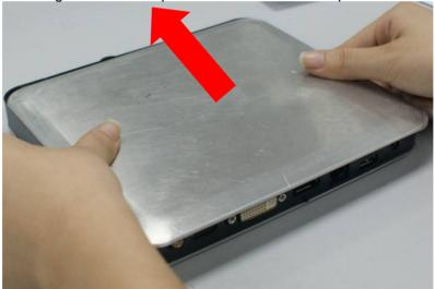
4. Put the side of I/O back panel towards you and push the removable cover of the chassis in the direction forwards.
