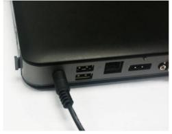
DC12V Jack: Connect the power adapter to DC12V jack after connecting connector power cord to adapter. Then Turn on the system either by power switch on front panel or remote control when all necessary configuration are made.
