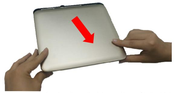
1. Put the side of I/O back panel towards you and push the removable cover of the chassis in the direction towards you. You can easily open the chassis only in the right direction.
