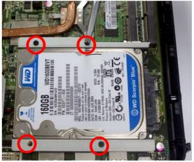
Lock the racks to the board by tightening up the screws in the marked position with a screwdriver.
