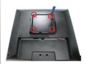
monitor by tightening up the screws in the marked position.
