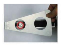
Lock the stand to the chassis by tightening up a screw to the marked place.
