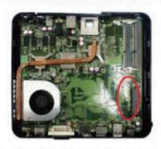
Locate HDD connector on the motherboard as the photo shows.
