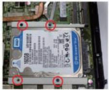
6.Lock the racks to the board by tightening up the screws in the marked position with a screwdriver.
