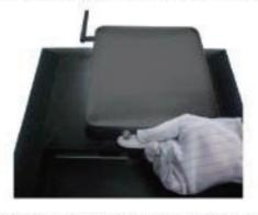
Lock the chassis to the rack by tightening up the screw in the marked position.
