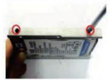
Lock the SATA hard disk to one of the racks by tightening the screws in the marked position.
