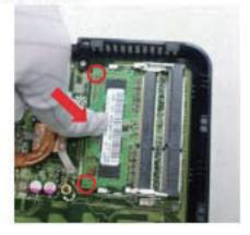
Press down as the photo shows. The eject tabs will lock it if installed correctly.
