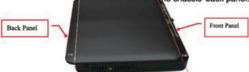
3.Place the removable cover upon the chassis. See to it that the left and right edges of the cover should be parallel to those of the chassis and there should be a distance of about 1 cm left between the front edge and the front panel of the chassis as the photo shows.
