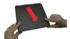
1.Put the side of I/O back panel towards you and push the removable cover of the chassis in the direction towards you. You can easily open the chassis only in the right direction.
