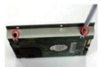
Lock the SATA hard disk to the other rack by tightening the screws in the marked position.
