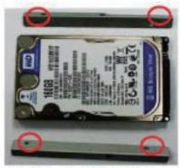
2.The SATA hard disk and the hard disk racks (see to it that the marked screw holes on rack and the corresponding holes on both edges of HDD).
