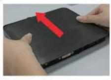
4.Put the side of I/O back panel towards you and push the removable cover of the chassis in the direction forwards.
