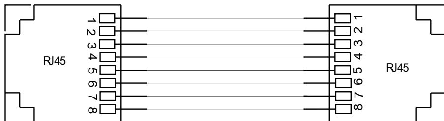
Fig.A-2 Order of Straight-through Cable
