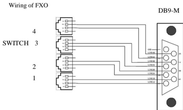
Figure 4-14 KODT3000 - SLC/SLR Wiring Figure
