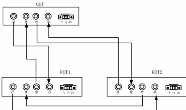
Figure 4-20 KODT Series Products Fiber Optical Connect
