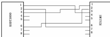
Figure 4-18 KODT3000 wiring for Ethernet 10Base-T
