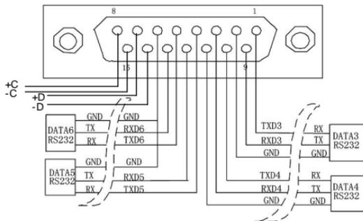
Figure 4-12 KODT3000B Series Products DATA2 wiring
