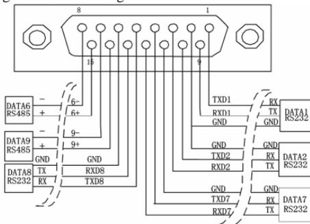
Figure 4-3 KODT3000 wiring of data int interface
