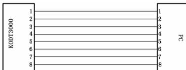
Figure 4-19 KODT3000 wiring for Ethernet 10Base-T
