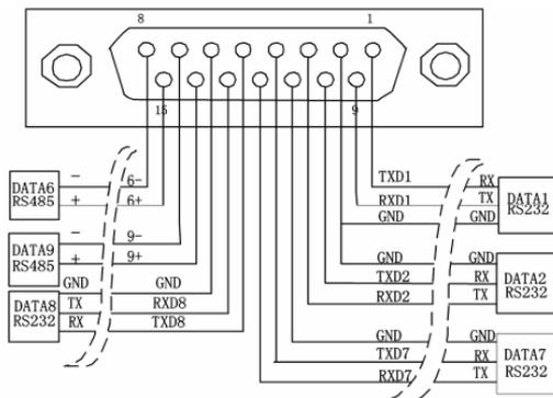
Figure 4-11 KODT3000 Series Products DATA1 wiring
