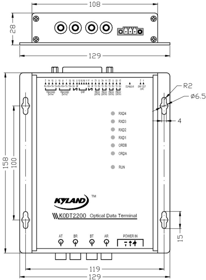
Figure 5-1 wall mounting dimension
