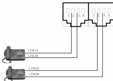
Figure 4-16 KODT3000 - SLR Wiring Figure
