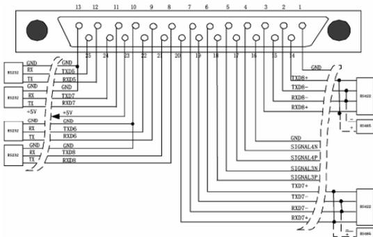
Figure 3-8 KODT2200B DATA2 wiring
