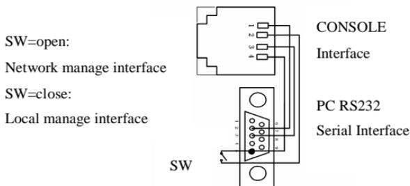
Figure 3-9 KODT2200 wiring of network manager
