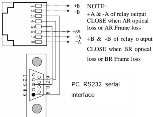
Figure 4-17 KODT3000 wiring of manager cables
