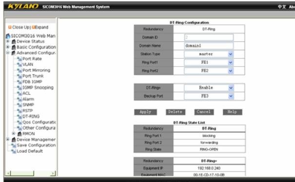
Figure 7-36 DT-Ring configuration state
